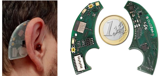
**Fig. 1.** The PrimeHA development platform for hearing aid algorithms, taken from [2].
